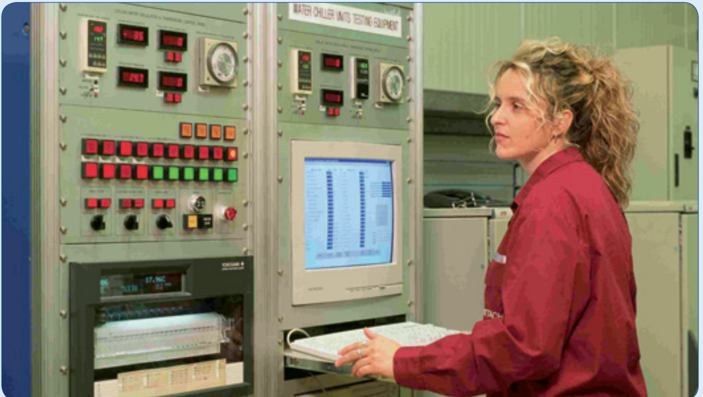
A computer system controls the results of the Commercial Test, obtaining in real time all the system variables and checking the correct operation of the unit.
